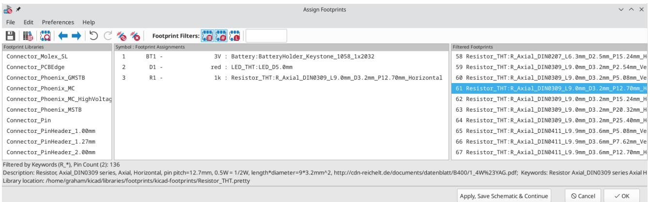
Many footprints are included with KiCad, so the footprint assignment tool offers several ways to filter out footprints that aren't relevant to the symbol in question.
