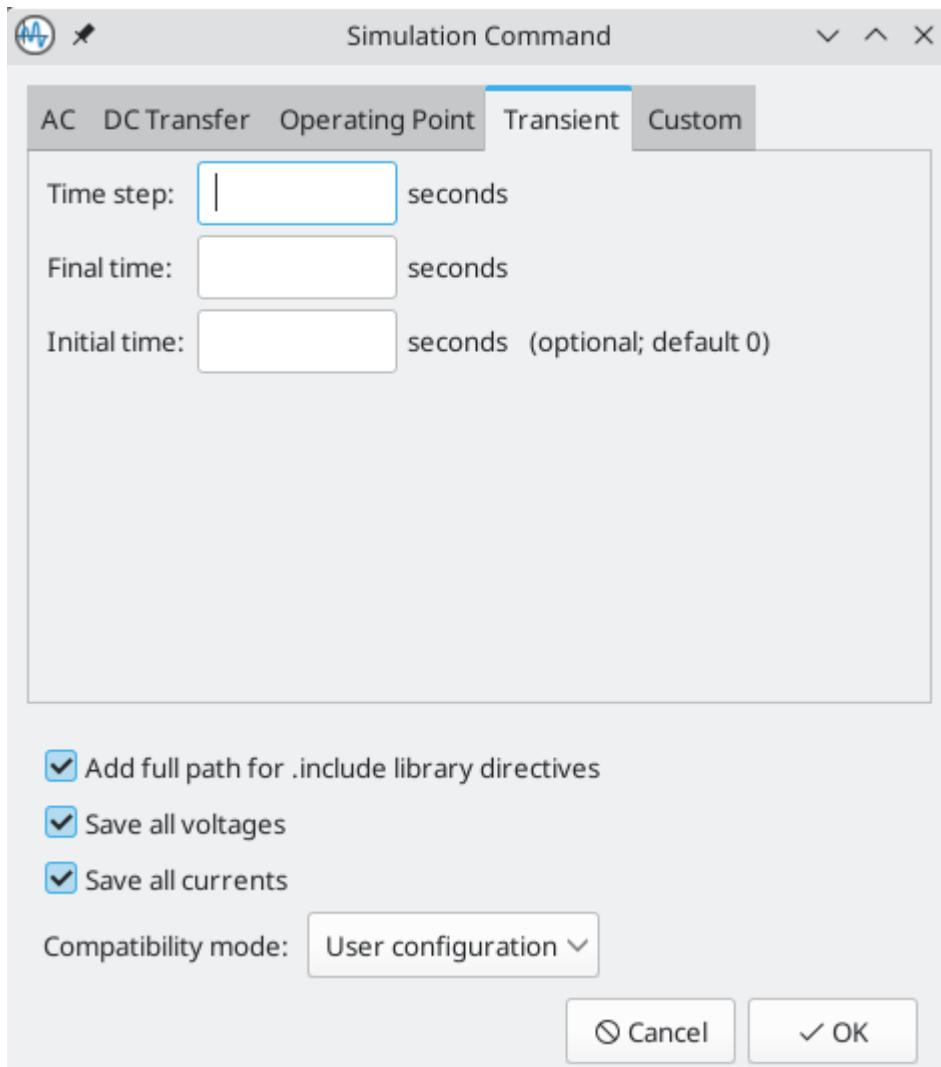
Calculates the time-varying behavior of the circuit.
