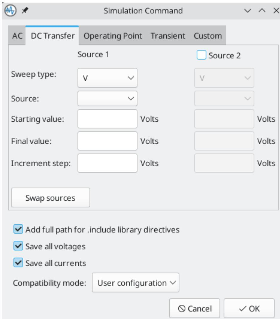
Calculates the DC behavior of the circuit while sweeping one or more parameters: source values (voltage or current), resistor values, or the simulation temperature.
