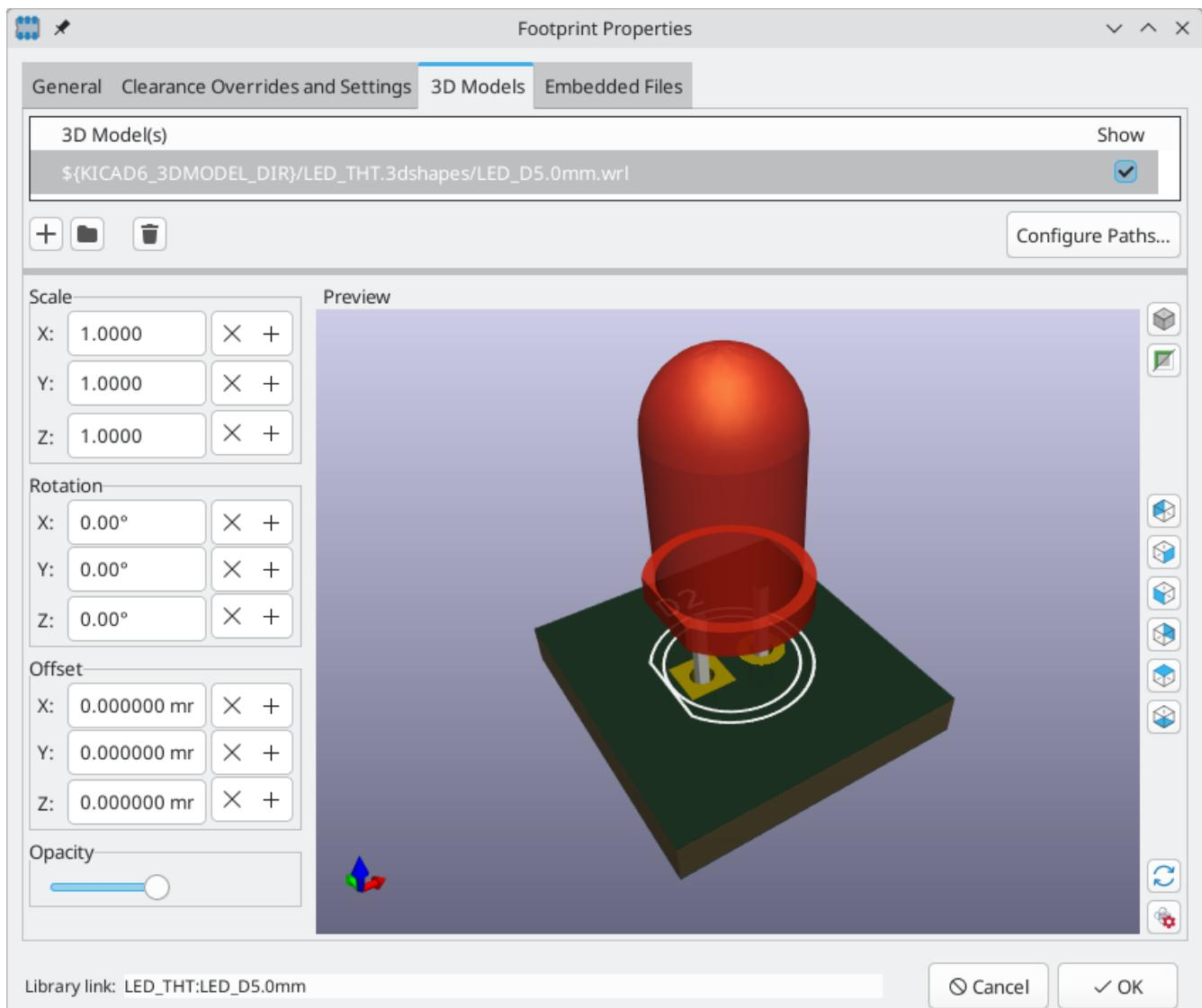
Both STEP (.step) and VRML (.wrl) 3D model formats are supported. STEP files are useful where dimensional accuracy is needed, while VRML files can be used for more visually attractive renders. Many footprints in KiCad's library have associated 3D models; these models are provided in both VRML and STEP formats. Only one of the two models needs to be listed in the footprint (typically the VRML filename is
